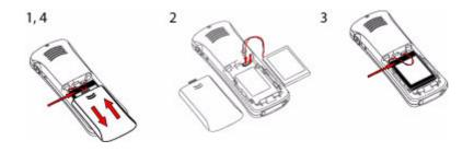
Figure 10:Battery replacement
